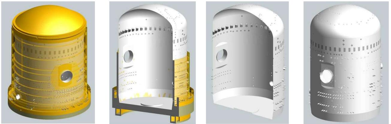
**Figure A.3.4:** 3D view of the liner for the reactor building containment, with the liner metal illustrated in grey and the reinforced concrete in orange
